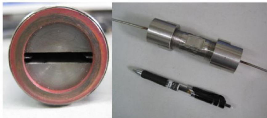
Figure 2.3 : Micro channel reactor : (a) Multi coil type (Izquierdo et al., 2012), (b) Radial pin hole type (Liu et al., 2012).
