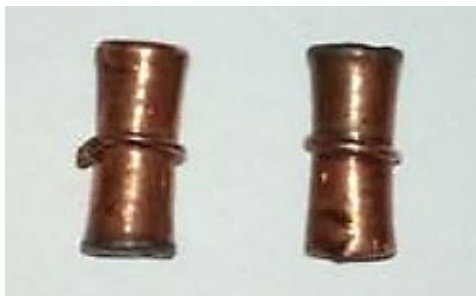
Figure 1.3: Electrode fabricated by FDM (Equbal et al. , 2017)
