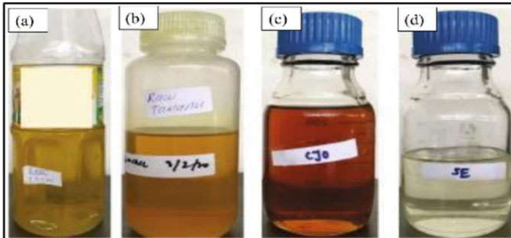
Fig. 1 MQL lubricant sample; a RBDPO, b CTO, c CJO and d SE
