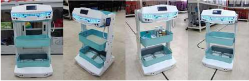
Fig. 4 The delivery robot's prototype body design
