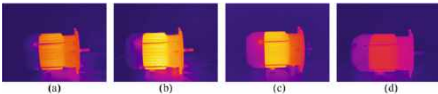
Fig. 1 Examples of thermal images from the dataset. a Is an image with 50% short circuit in one phase of stator. b Is an image with 50% short circuit in 2 phases of stator. c Is image with blocked-rotor and d is image with blocked fan
