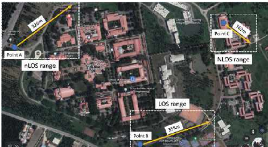
Fig. 2 Radio transmission coverage radius and testing points
