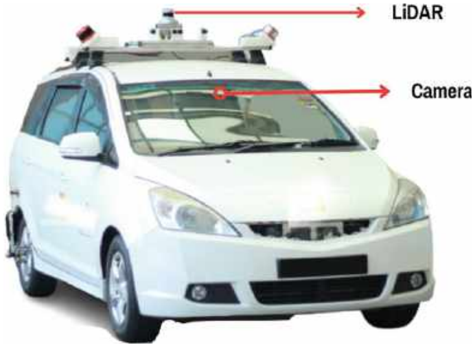
Fig. 2 The position of the camera and LiDAR at the host vehicle
