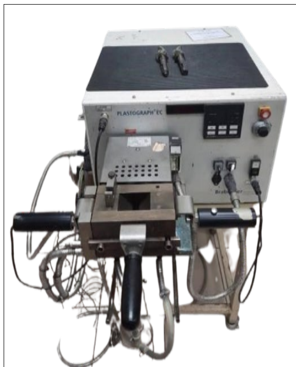
FIGURE 1. Brabender plastography machine for blending PHA/nCaP/chitosan biocomposite.
