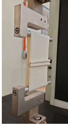
FIGURE 1. Looped fabric sample mounted on looped bar of tensile machine.
