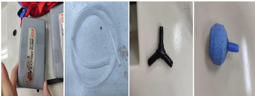
Figure 4. Aquarium battery pump (portable), tube, pipe distributor and air stone mineral
