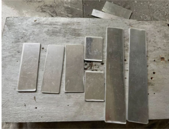
Fig. 2 The result of an aluminum sheet after being shaped using grinder during fabrication
