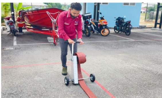
Fig. 5 The testing process of hose roller at Pagoh fire station
