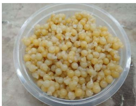
(c) Ceramic chitosan beads after 12 hours
