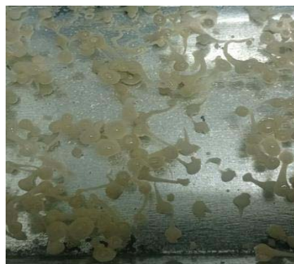
(b) Ceramic chitosan beads in NaOH solution
