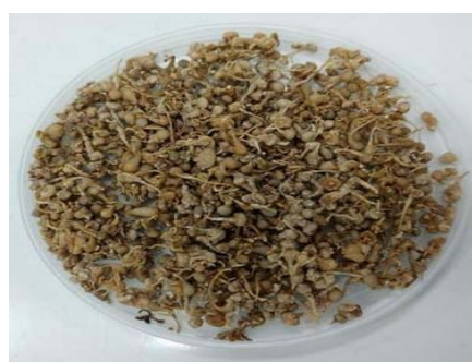
(d) Ceramic chitosan beads after drying in an oven at 100 within 1 hour
