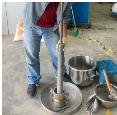
Figure 1. Compaction test in a standard proctor mould by using 4.5 kg hammer.
