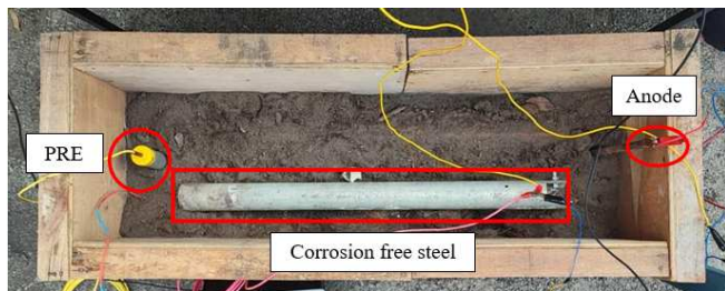
Fig. 6. The experimental and measurement setup
