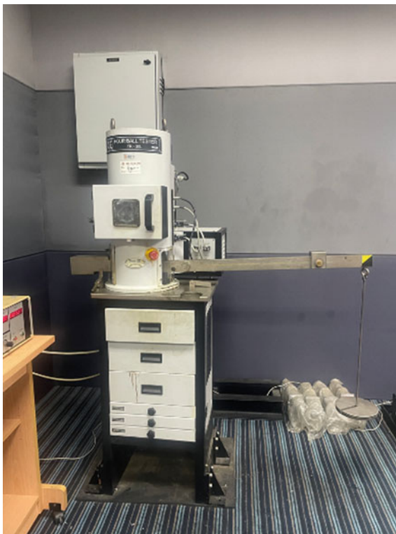
Fig. 2 Four ball tribotester machine
