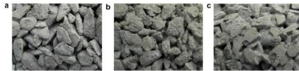
Figure 11. Effect of cement flow on surface shapes of PC and sound absorption properties[36]
