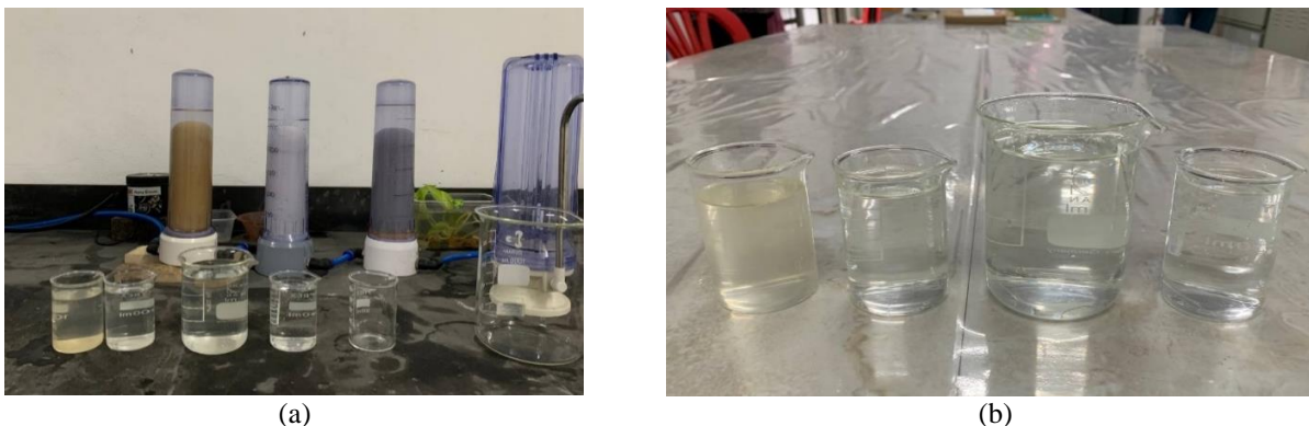
FIGURE 4. Demonstration of the water filtration system by 60wt.% of silica water filter
