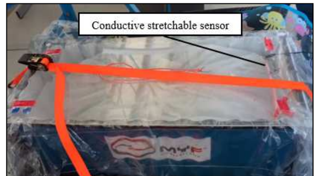
Fig. 6. The conductive stretchable sensor installation.
