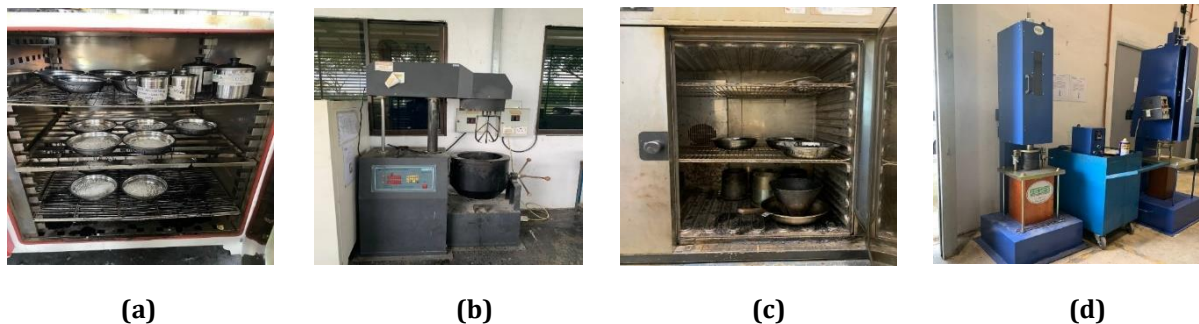
Fig. 2 Marshall mix design preparation (a) Heating material; (b) Mix material; (c) Heating loose specimen. (d) Compaction machine
