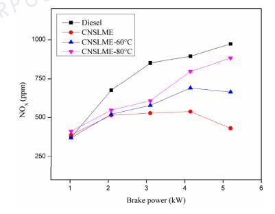
Figure 2.6: Effect of fuel preheating on NOX emission [37]
