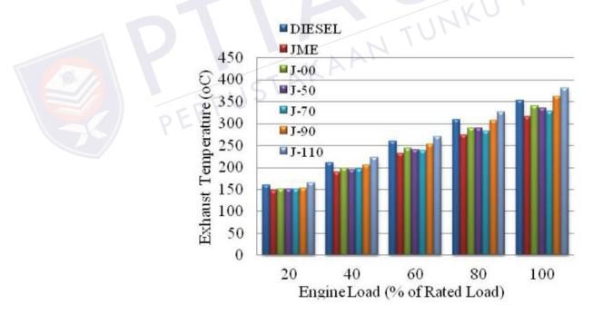
Figure 2.5. Variation of Exhaust gas temperature with load at elevated fuel inlet temperatures [35].
