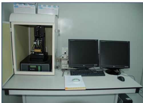
Figure 3.16: Image of the Park System AFM (model XE-100) operation system.
