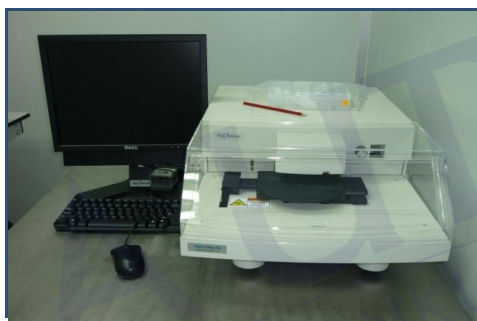
Figure 3.12: Surface profiler Alpha Step IQ.
