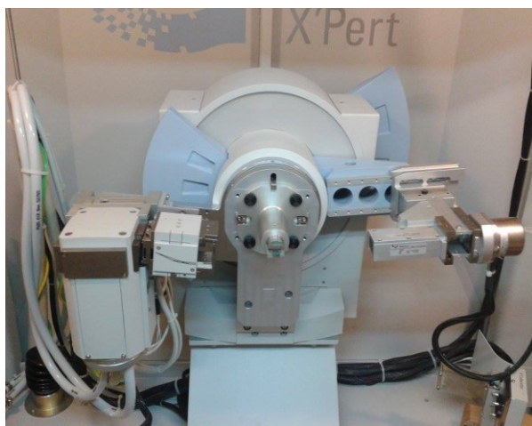
Figure 3.19: Picture of the Panalytical X'Pert Pro-MRD used for the measurement.
