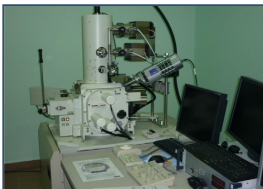
Figure 3.14: Image of the FESEM (JEOL JSM-7600F) operation system.
