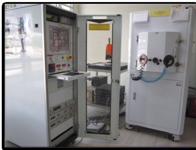
Figure 3.6: Overview of RF magnetron sputtering setup.
