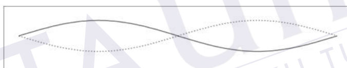
Figure 2.5: The two halves of the string vibrate in opposition each other
