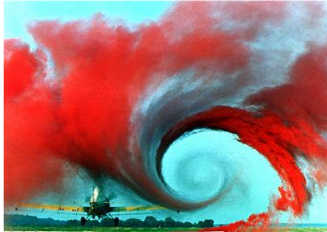
Figure 2.1: Vortex created by the passage of aircraft wing, which is exposed by the colored smoke (Rafiuddin, 2008)
