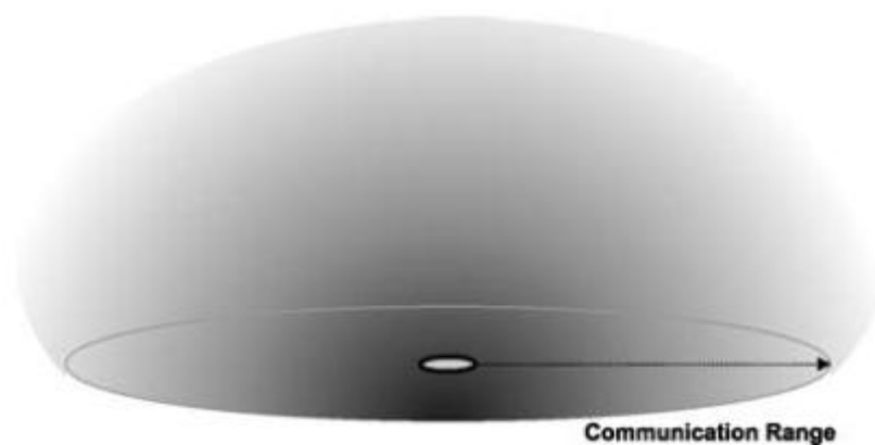
Figure 2.7: Decreasing signal transmitted by a transmitting node. The signal is send with specific signal strength which decreases as the square of distance. In real world different other factors also contribute in decreasing signal strength (Boukerche, 2009)
