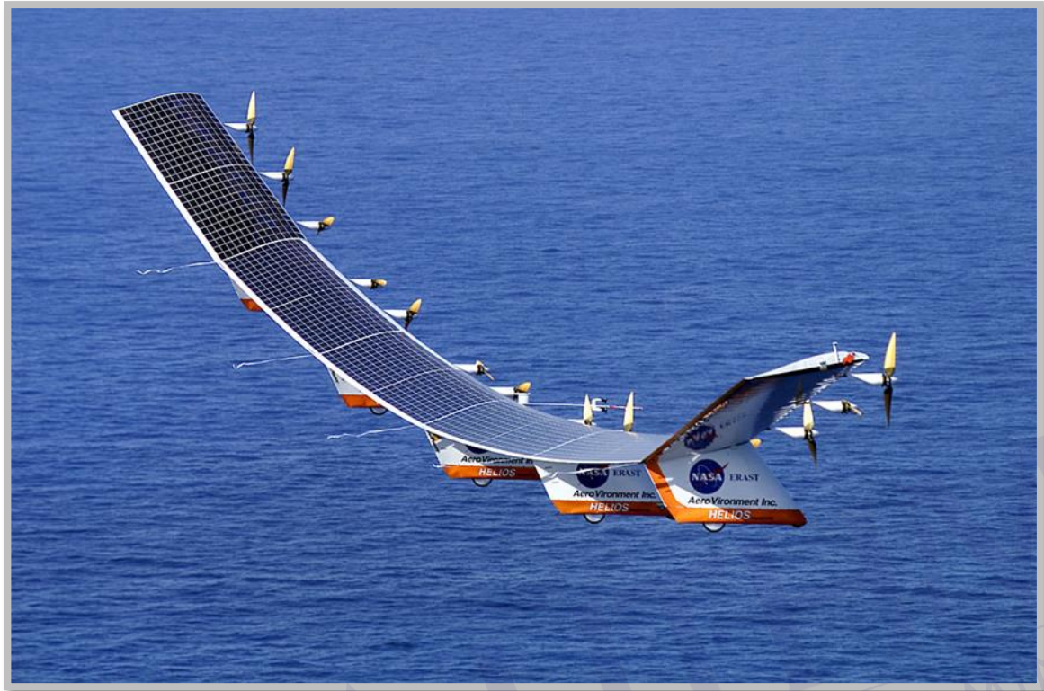
Figure 2.2: Solar-powered unmanned aircraft [5]
