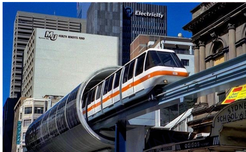
Figure 2.1: Sydney Metro Monorail in Australia singular (mono) beam, with a train wider than guideway. [2]
