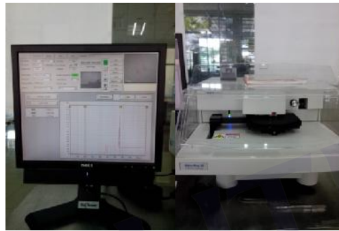
Figure 2.10: Surface profiler taken from MiNT-SRC, UTHM
