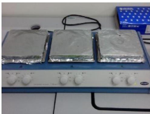
Figure 2.4: Magnetic stirrer taken from MiNT-SRC, UTHM
