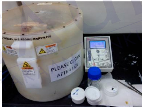
Figure 2.3: Spin coater taken from MiNT-SRC, UTHM
