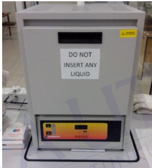
Figure 2.6: Annealing chamber taken from MiNT-SRC, UTHM
