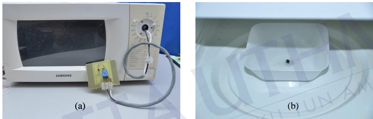
Figure 3.2: Setup for microwave oven. (a) Relay circuit replaced the oven timing switch, (b) Tray with temperature sensor on oven cavity.
