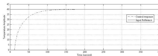
Figure 12. Response of physical model with FPD controller
