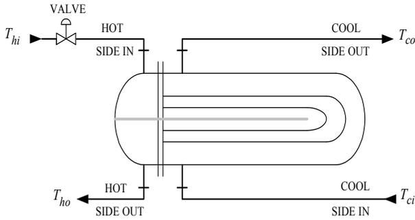
Figure 2. Shell and tube heat exchanger input output
