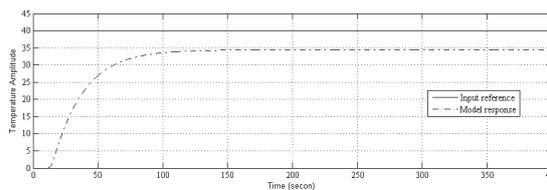
Figure 13. Response of system identification model with FPD controller
