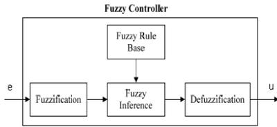
Figure 5. Fuzzy logic block diagram
