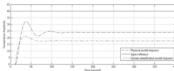
Figure 11. Comparison of two models response without controller
