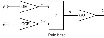
Figure 6. FPD controller block diagram
