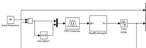
Figure 8. Matlab Simulink block control system for model from non-parametric system identification
