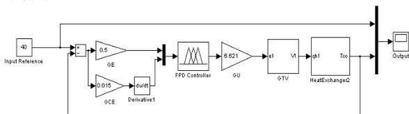
Figure 7. Matlab Simulink block control system for model from dynamic modeling
