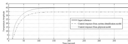
Figure 14. Comparison of two models response with FPD controller
