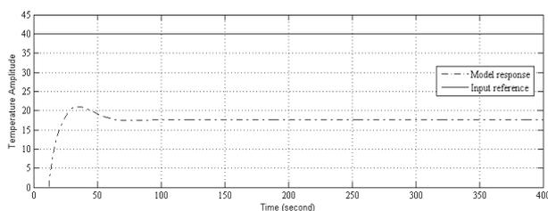
Figure 9. Response of physical model without controller
