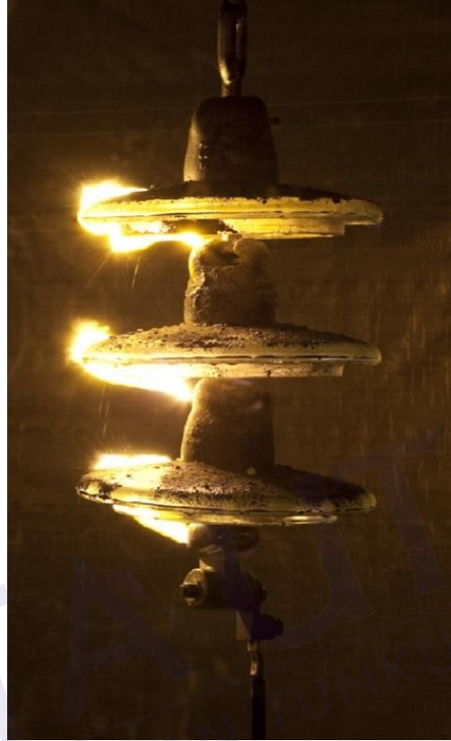
Figure 2.5: Flashover in HV insulator equipment or called “corona discharge” [12]
