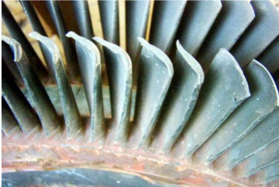
Figure 2.1: Deformed Turbine Blades Under Creep Attack. [4]
