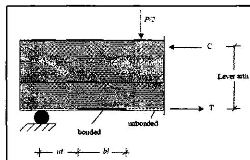
Figure 3: Bonded and Unbonded Lengths (Lorenzis and Nanni, 2000)
