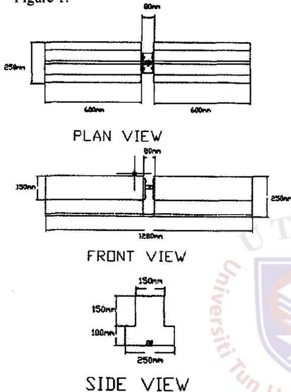
Figure 1: Block Dimensions
