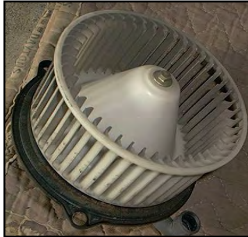
Figure 2.7 : Squirrel cage that used to help move air throughout the passenger compartment.
