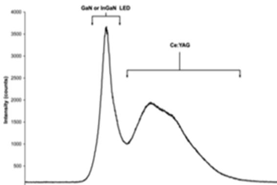
Fig. 5: The Spectrum of White Light LED
