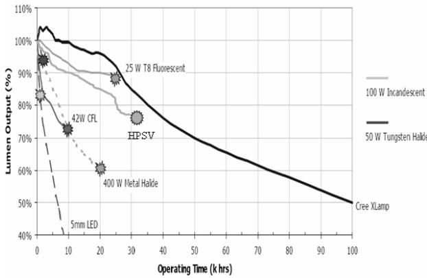
Fig. 1: Lumen output performance of several lighting sources
