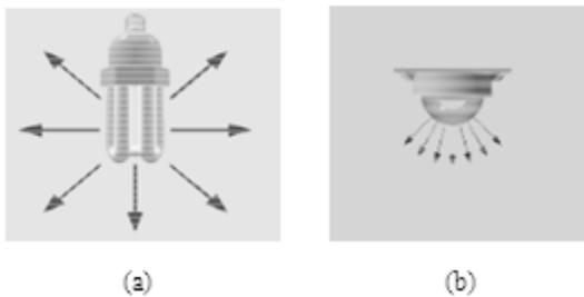
Fig. 2: The output light (a) Conventional lamp (b) LED
