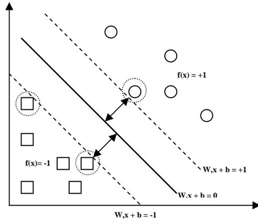
**Figure 1: SVM classification example for separable two classes.**
