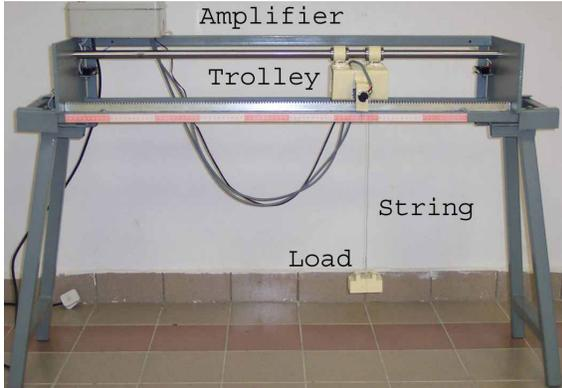
Figure 1: Lab-scale gantry crane
