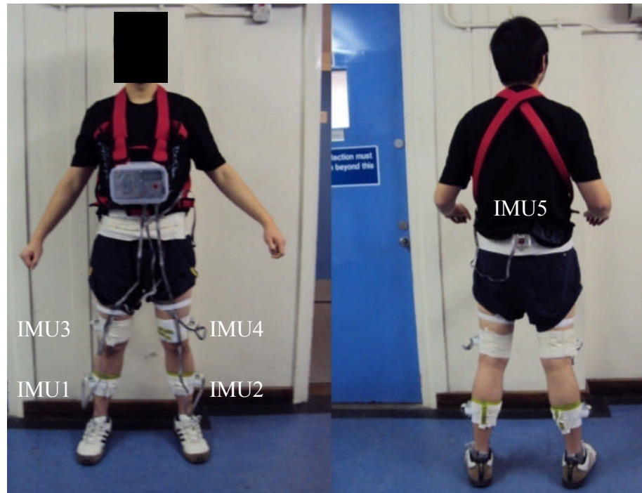
Figure 5.3: The body landmarks and the IMUs
