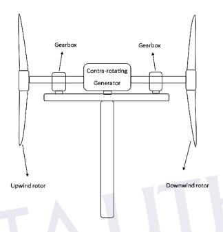
Figure 1.1: Typical counter-rotating HAWT
