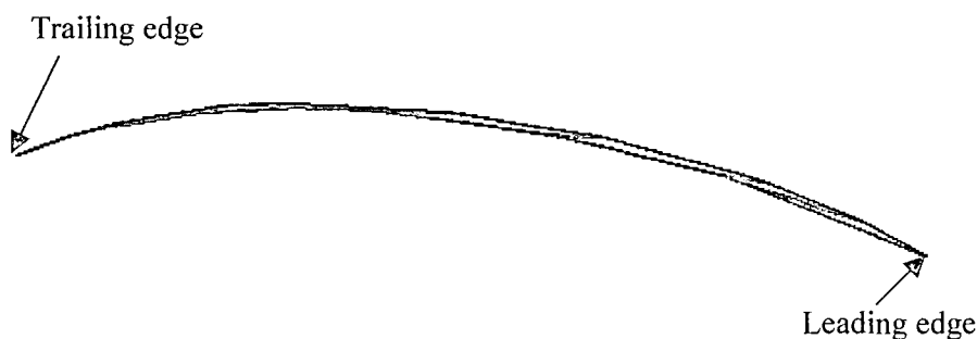
Figure 2.1: The top view of AE2 blade shows its airfoil section
