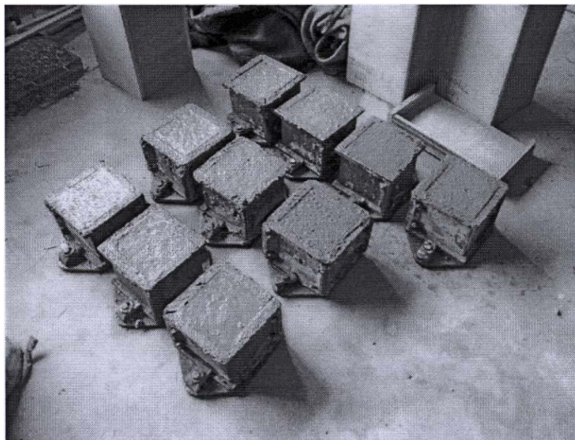
Figure 3.2 The cubes cast for the cube tests
