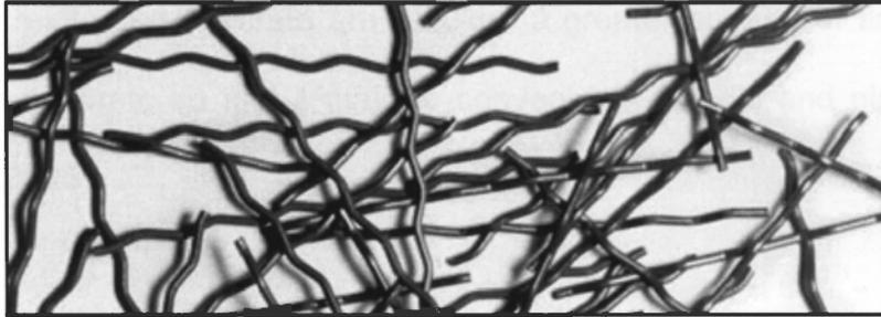
Figure 1 steel fiber type Undulated
