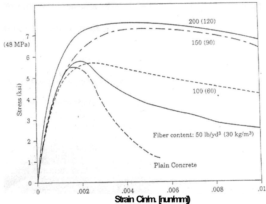
Figure 6 the Stress strain behavior of steel fiber for normal concrete strength containing 50 mm hooked end.
