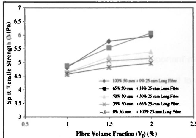
Figure 9 Split tensile strength of fibrous concrete with mixed aspect ratio of fibres at different fibre volume fractions by Y. Mohammadi et al 2008
