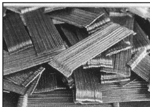
Figure 4 (b) Type of steel fibers used in this research
