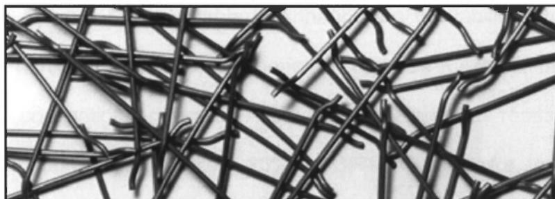
Figure 2 steel fiber types flat
