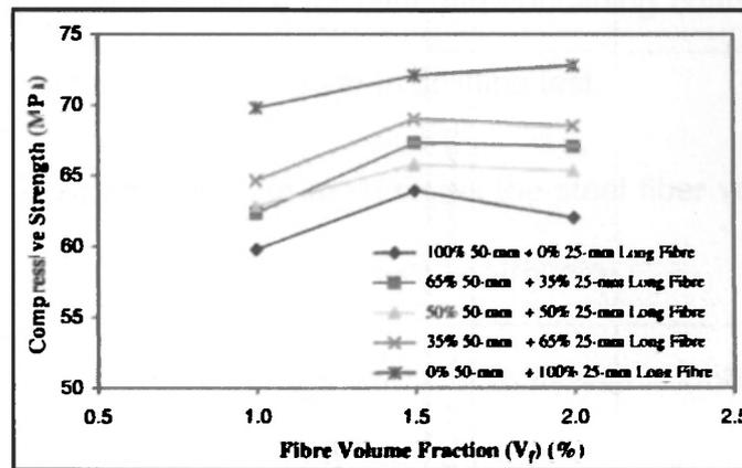
Figure 8 Cube compressive strength of fibrous concrete with mixed aspect ratio of fibres at different fibre volume fractions by Y. Mohammadi et al 2008
