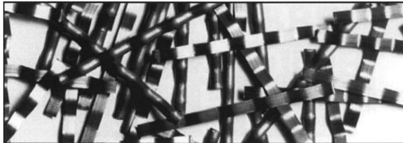
Figure 3 steel fiber type Hooked
