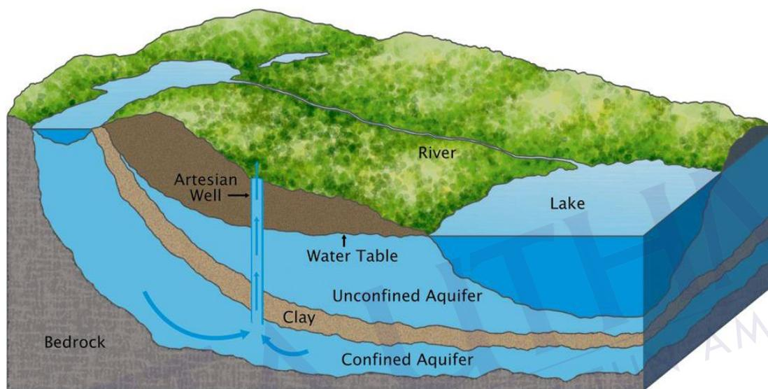
Figure 2.2: Schematic representation of Groundwater aquifer (Gunther, 2011)
