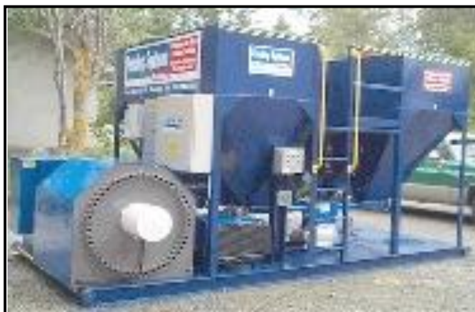
Figure 2.4 : Centralized Feeding System (Dirfeeders, 2005)
