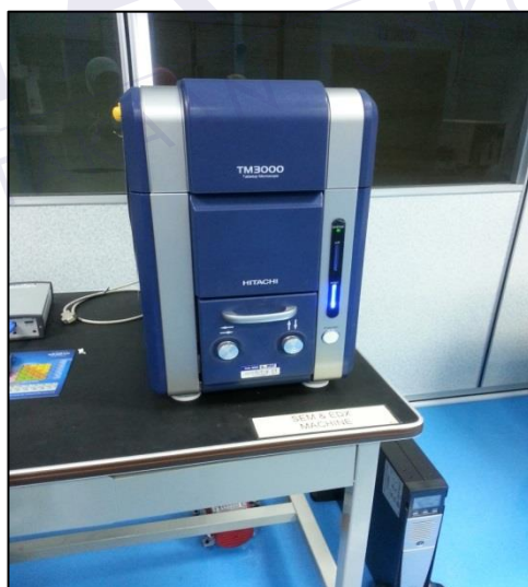
Figure 4.3: SEM with EDX: TM3000 Hitachi at UniMAP
