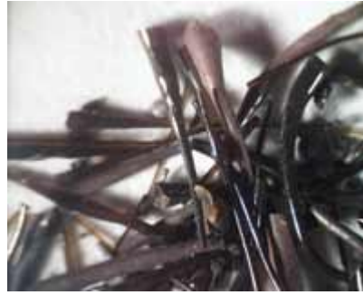
Figure 2.4: Boiler Slag 'Needles' as viewed via a microscope
