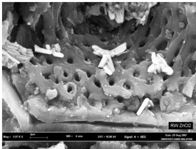
Figure 2.1: Scanning Electron Macrographs for The External Morphology Of The Activated Carbon At The Pyrolysis Temperature of 500°C.
