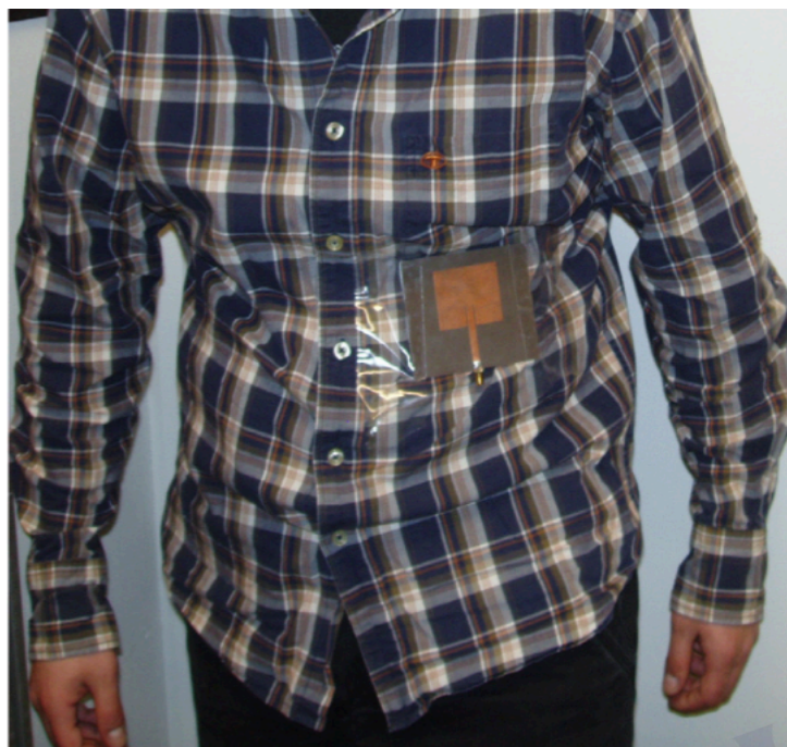
Figure 2.8: Microstrip patch antenna attached on chest [26]
