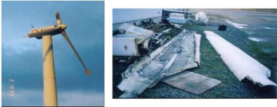
Figure 2.2: Damage of wind turbine blades due to lightning[7]
