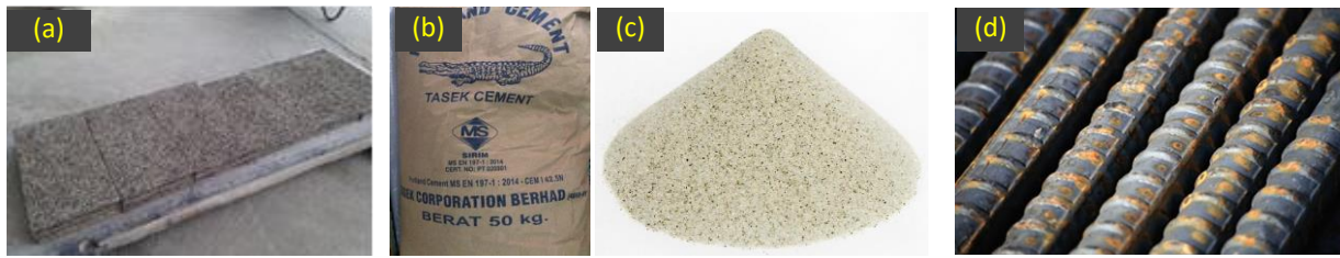
Figure 5. (a) 50 mm thickness of WWCP (b) Portland cement (c) Fine sand (d) High yield steel bar
