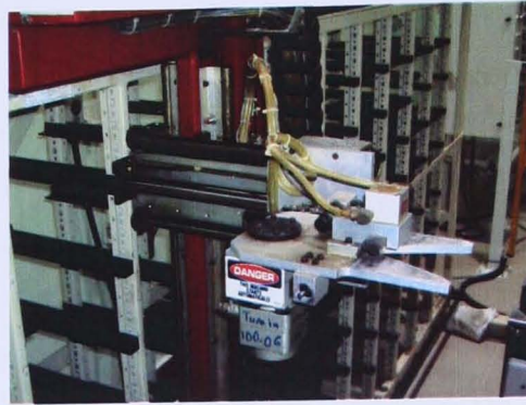
Figure 3.6: The SRM pneumatic end-effectors for storing/retrieving
