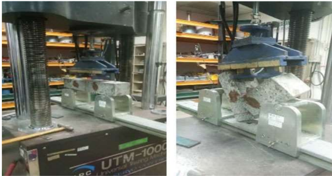
Fig. 1 Flexural test setting up (left) and sample testing (right)
