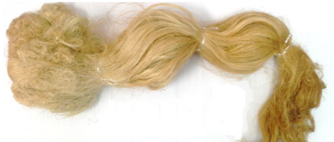
Figure 1. The appearance of the PALF fiber after the extraction process.
