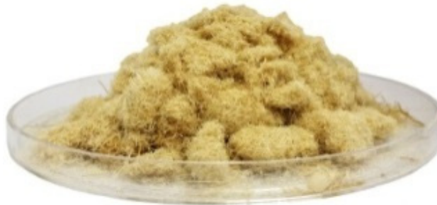
Figure 2. The physical of the PALF fiber after the crushing process.
