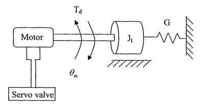
Figure 1.1 : Physical model of nonlinear electrohydraulic servo control system
