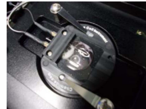
Figure 1. Picture of 9mm – gap EP electrode chamber for \mu sPEF excitation.
